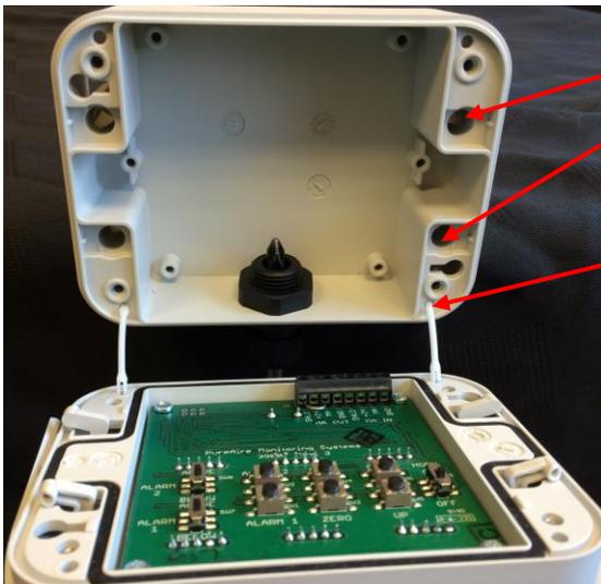
signal from your oxygen monitor, pushing these switches will automatically adjust the zero and full scale readings on the Remote Digital Display.
